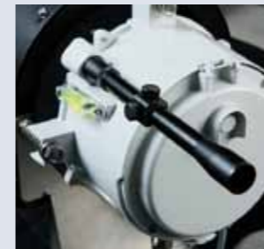
Precision alignment A gun sight can be utilized for precision alignment to the center line of the range.
